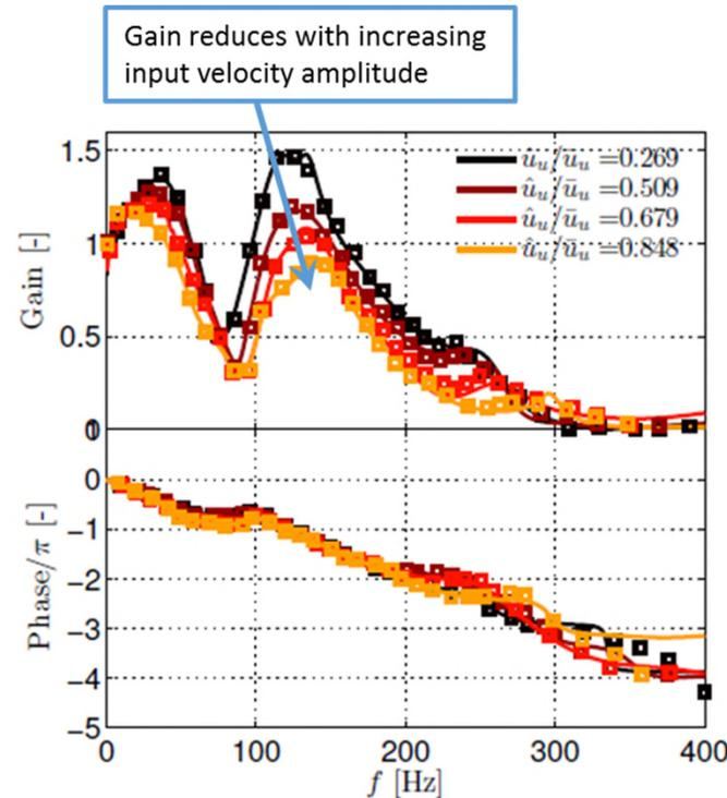
Flame describing function results for a gaseous fuelled test combustor.
