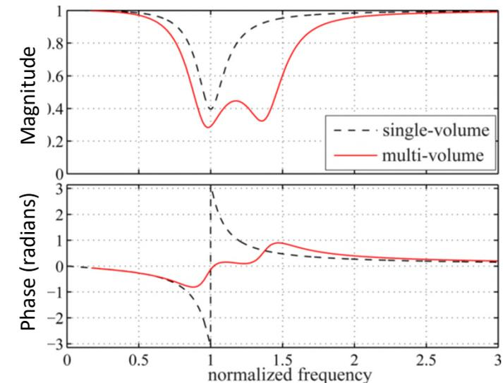
Reflection coefficient from: Bothien et al., A Novel Damping Device for Broadband Attenuation of Low-Frequency Combustion Pulsations in Gas Turbines, Journal of Engineering for Gas Turbines and Power, APRIL 2014, Vol. 136
