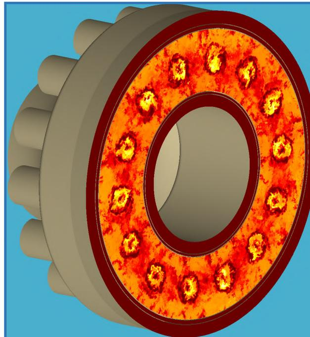
Solar 14 burner GT combustion system fully modelled using LES
