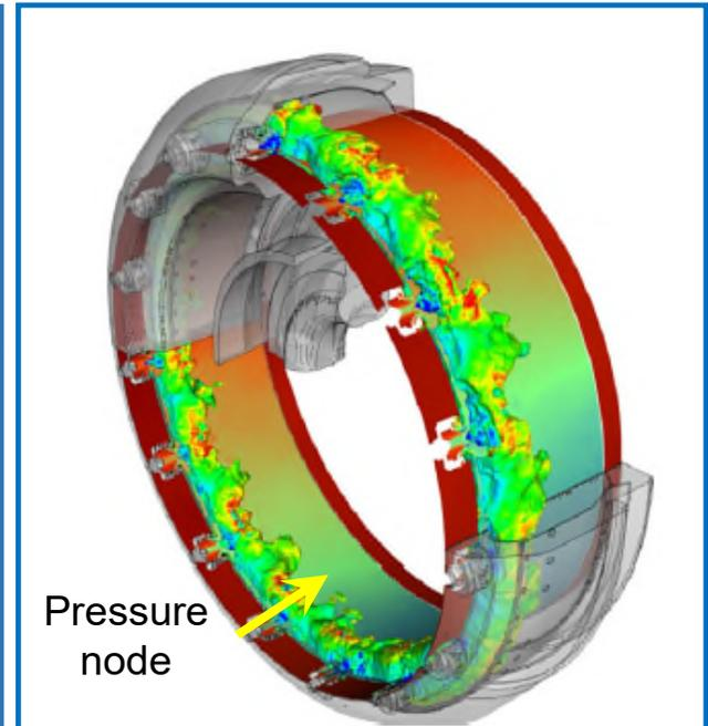
LES of the first azimuthal unstable mode in an helicopter engine: pressure on a cylinder passing through the burner axis and iso-surfaces of temperature coloured by axial velocity (
