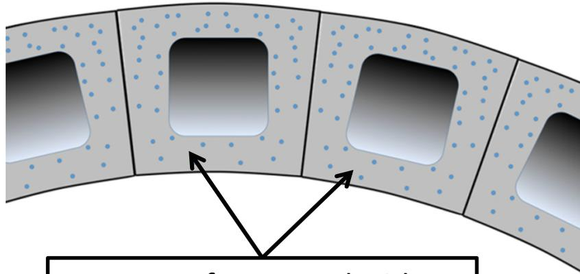
Burner front panel with multiple resonator necks/purge air holes.
