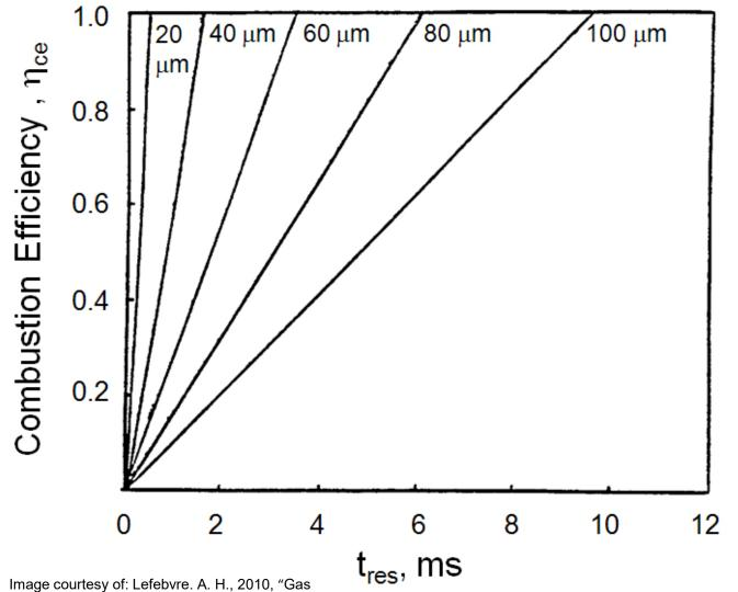
Influence of fuel mean drop size on evaporation ratecontrolled combustion efficiency (Fuel: Diesel Oil)
