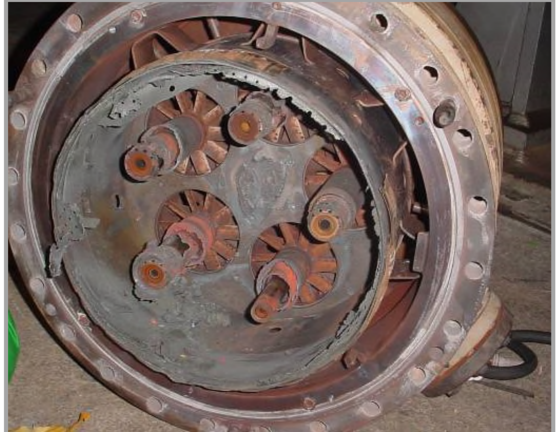
Damage following mechanical failure due to high frequency dynamics ( \sim 2\text{kHz} ) which can be linked to fuel changes
