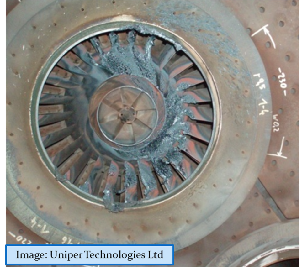
Damage as seen here has been attributed to flashback due to high levels of C2+
