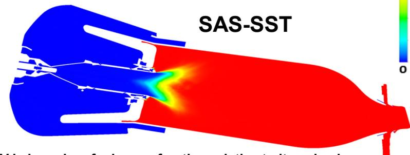
PV is based on fuel mass fraction relative to its value in both reactants and products
