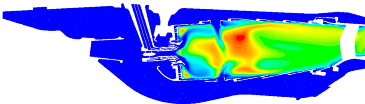
High fidelity CFD Model of a Typical Annular Combustion System
