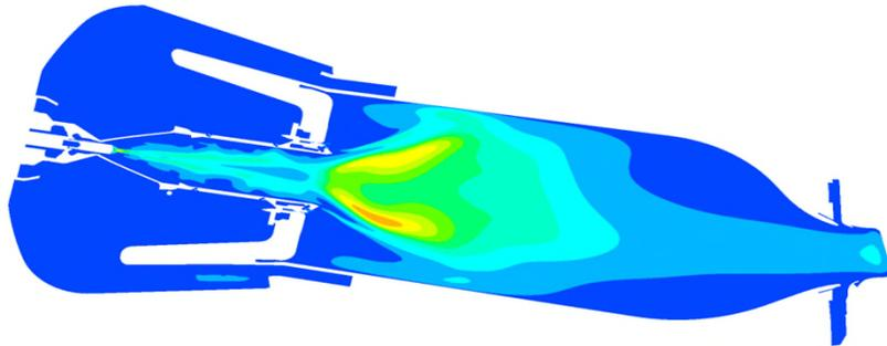
**Turbulent kinetic energy****SAS k- $\omega$  SST
