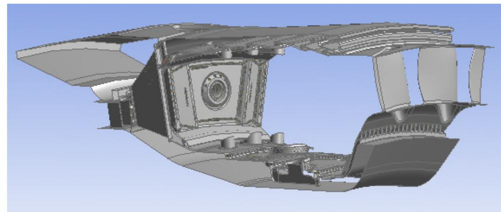
Injector details, Liner cooling details, Exit Guide Vanes...
