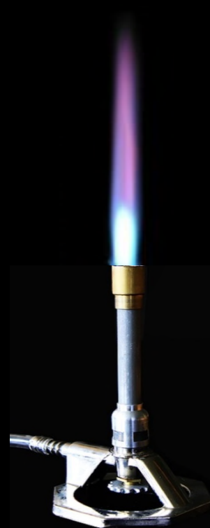
Partially Pre-Mixed Flame (more pre-mixing)
